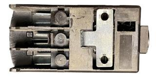
Technical data: Rated insulation voltage: 400V Rated current: 16A Rated connecting capacity: 2.5mm2 Rated ambient termperature: 125 drgee Model No.: BL503 Metal Parts: Q235-a Iron, surface plating Zinc. Note: this terminal is only designed for flexible cable IP: IP30
